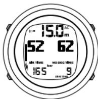
The change in your air consumption is based on constant one second interval pressure measurements over periods of 30–60 seconds. An increase in air consumption decreases the remaining air
