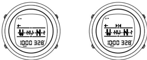
If, at any point, your bearing moves outside the compass display, right or left arrows appear to show turn direction.
