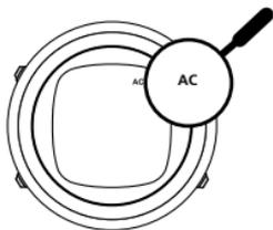
The **AC** is shown until the water contact deactivates. It is important to keep the water contact area clean. Contamination or dirt can prevent automatic activation/deactivation.
