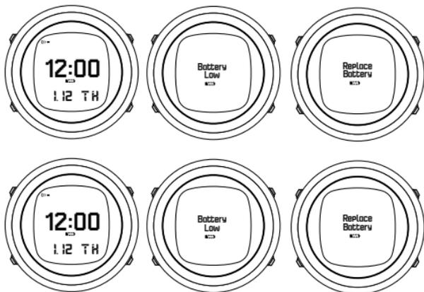
If the low battery icon appears in surface mode, or if the display looks faded, the battery may be too low. Battery replacement is recommended.
