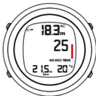
When the maximum allowed ascent rate is exceeded, the lower segment of the bar starts to blink and the top segment stays solid.
